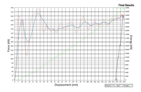
Measured Energy Output: 37.8 [kJ]Peak Displacement: 149 [mm]
