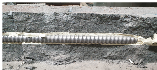
Figure 7. A cross sectioned sample of a resin anchored element following dynamic testing.
