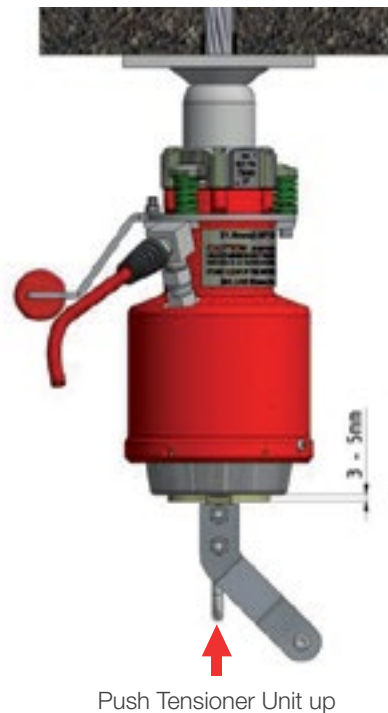
Figure 2. Fitting the Tensioner Unit to a Cable Tail
